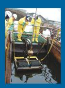
The oil skimming technology developed by Victoria Broje when she was a doctoral student at UCSB?s Bren School of Environmental Science & Management was put to work in the gulf. Broje came up with a new design for skimmers that use rotating drums to collect floating oil. By adding grooves to the drum surfaces, Broje, who now works for Shell Projects and Technology, made them much more efficient at collecting oil.
